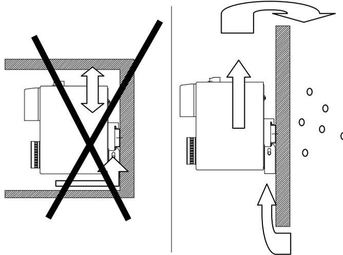
The converter must be mounted vertically (power block X6 above).
