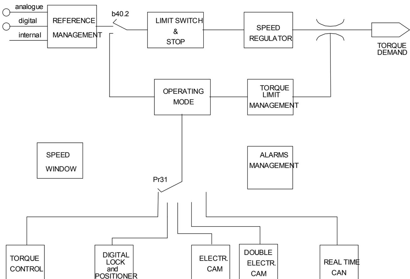
The main block diagram and the diagrams for special functions (operating modes) are described later in more detail.
