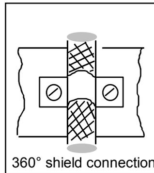
In general the shield should be connected at each extremity. In certain circumstances, however, control cable shields may be connected only at one end to eliminate mains hum that could interfere with the control signal. Decide case by case as numerous factors must be considered. Adopt the following general approach: if the screen is solely for shielding, connect at both ends. If current flowing in the shield interferes with the shielded signals, connect at one end only.
