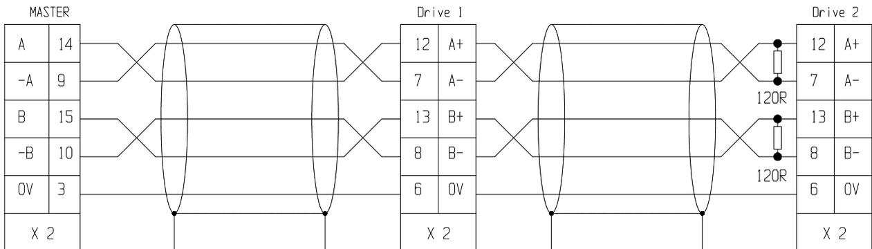
In the example given above, the connection of two SLVD-N to the Digital-Lock with a master is shown, but the diagram could be extended to several converters respecting the series connection. The line charge resistors must be connected to the last converter. The master can be an encoder powered externally or an encoder simulator of another converter.
