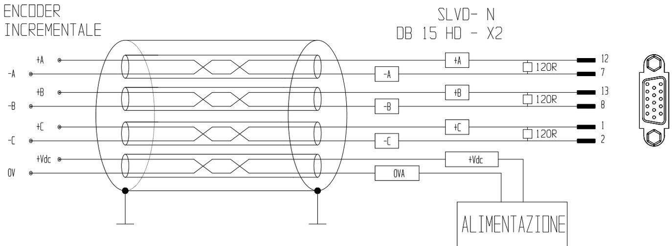
The second input in frequency is on the X4 connector, digital inputs. The input can receive signals in quadrature and frequency/sign, (b42.4), from IN2 and IN3 digital inputs. Follow the outline of connection:
